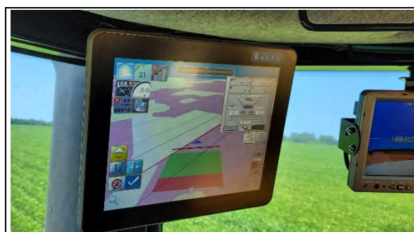
Figure 4. A variable rate fertilizer prescription plan on a display in the cab of a self-propelled fertilizer spreader as it travels through the field. This prescription plan was developed using image analysis of drone imagery in a Clemson University and USC-Aiken project supported by the SC Soybean Board.
