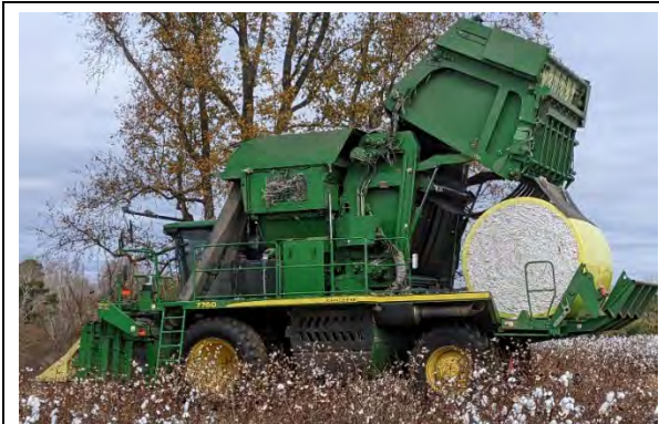
Figure 10. RFID enabled cotton picker. Tags are embedded in the module wrap.
